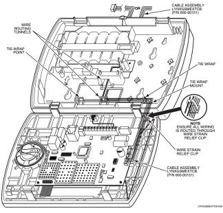
Figure 2. LYNX PLUS Cable Routing
